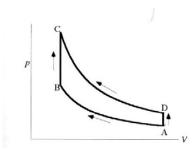
To see that W and Q are not state variables, note that one can move the system between two points A to C, each defined by specific values of state variables, via different paths. This is shown in the Figure, and one should compare paths through either D or B. The passage via different paths involves different amounts of work and heat transfer, but the total energy at the end is of course the same.
