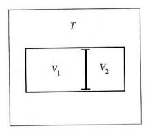
Consider now a small displacement of the piston such that  $V_1 \to V_1 + dV$ . Then  $V_2 \to V_2 - dV$ , and the change in free energy F is just
