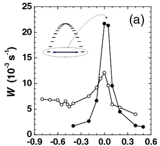
Fig 30: *The effects of decoherence. LEFT: A superconducting SQUID scans through different tunneling splittings, & ‘resonates’ with different environmental 2-state systems- disrupting its behaviour (Martinis et al, Santa Barbara). RIGHT: The nuclear spin environment entangles with a magnetic molecular spin, & its relaxation rate  $W$  is radically increased (Morello et al, Leiden)*
