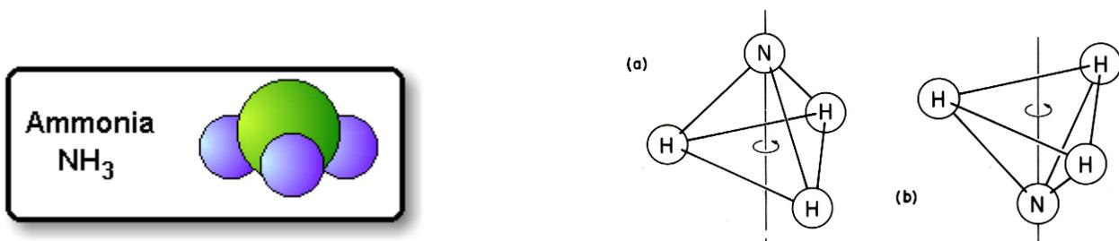
Fig 12: *The Ammonia molecule. LEFT: basic structure, with a Nitrogen atom above a triangle of Hydrogen atoms. RIGHT: The N atom can also lie below the  $\text{H}_3$  triangle, and tunnels between the 2 configurations (a) and (b).*
