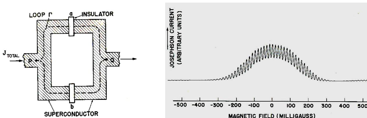
Fig 10: *The ‘SQUID’*. LEFT: schematic SQUID- electrons come in at left, travel through the 2 arms, via the insulating ‘Josephson junctions’ a and b, and out to the right. RIGHT: The current coming out of the SQUID as a function of the magnetic field through the SQUID.
