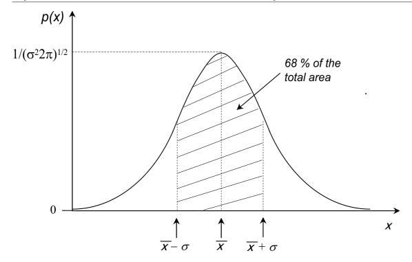
Figure 1: The probability density p(x) for a Gaussian distribution. The area under this function over some range of x gives the probability that x lies in that range. For instance, the total probability of x being within one standard deviation of the mean is 68 %
