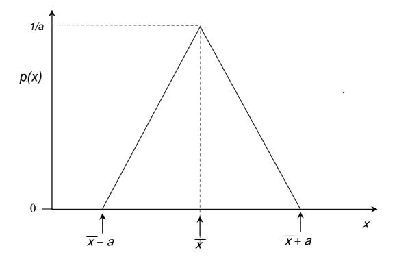
Figure 3: The probability density p(x) for an analog measurement. The reading on the scale is  $\overline{x}$ , which is also the mean value of the distribution. The maximum uncertainty estimated from the scale is  $\pm a$ . The value of p(x) within this uncertainty range is peaked at value 1/a, normalized so that the integral of the whole distribution is unity.
