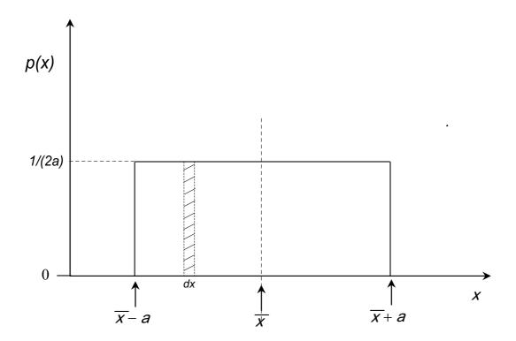
Figure 2: The probability density p(x) for a digital measurement. The reading on the meter is  $\overline{x}$ , which is also the mean value of the distribution. The maximum uncertainty due to rounding is  $\pm a$ . The value of p(x) within this uncertainty range is uniform and takes on the value 1/(2a) so that the integral of the whole distribution is unity.
