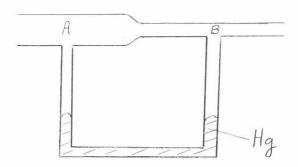
A glass tube is set up as shown on the left, with a mercury manometer attached at points A and B. The tube is circular with the diameter at A twice that at B. A flow of water, from A to B, is then started.
