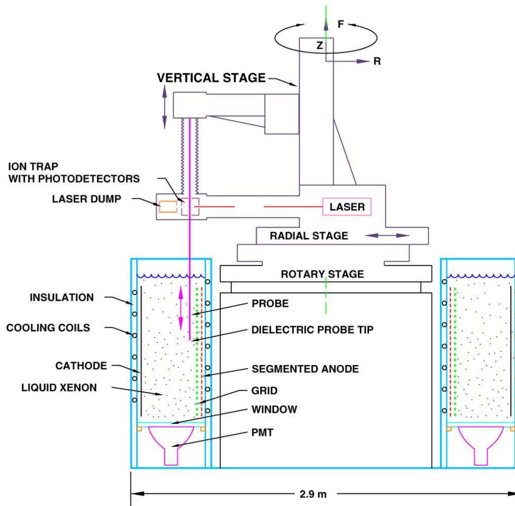
Look at 10 tonnes of  $^{136}\text{Xe}$  in a liquid or gas TPC. Use laser spectroscopy on the resulting ion to confirm it is barium, rejecting backgrounds. Sensitivity of  $\sim 10$  meV
