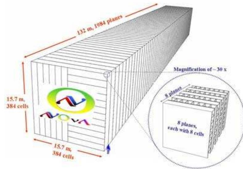
A 30 kton active scintillator detector with fine segmentation to see  $\nu_e$  appearance.
