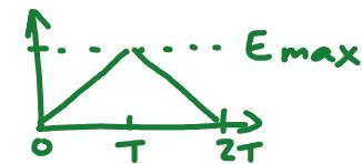
$$\text{So: } P(2T) = \frac{256}{81\pi^4} \cdot \frac{q^2 a^2}{\hbar^2} \cdot \left| \int_0^{2T} dt e^{i(E_2 - E_1)t/\hbar} E(t) \right|^2$$
