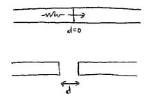
understand the tunnelling quantitatively. If d=0, the electron will definitely get to the second wire (probability 1). For a finite separation, we can estimate the tunnelling probability by how much the probability density for the electron's
