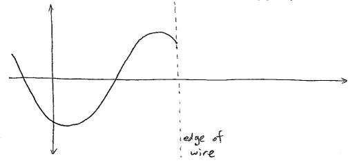
d) We can see that there is some probability of finding the electron outside the wire, even if its energy is less than the work function. What is the probability density for finding the electron at a distance d into the air gap, relative to (i.e. divided by) the probability density for finding it at the edge of the wire? Answer in terms of m,  $\hbar$ , W, E, and d.
