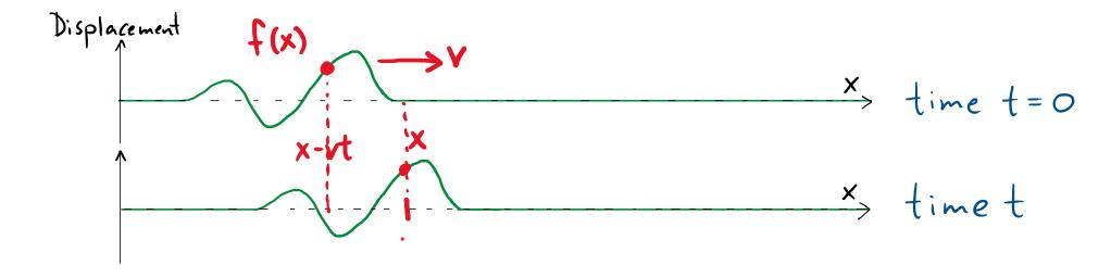
At time t=0, a right-moving wave pulse has displacement D(x,t=0) = f(x) shown in the top picture. At a later time t, the displacement will be described by
