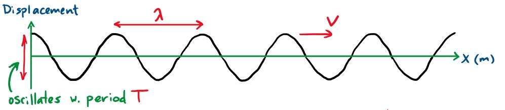
Right moving wave: D(x,t) = Acos(kx - wt)
