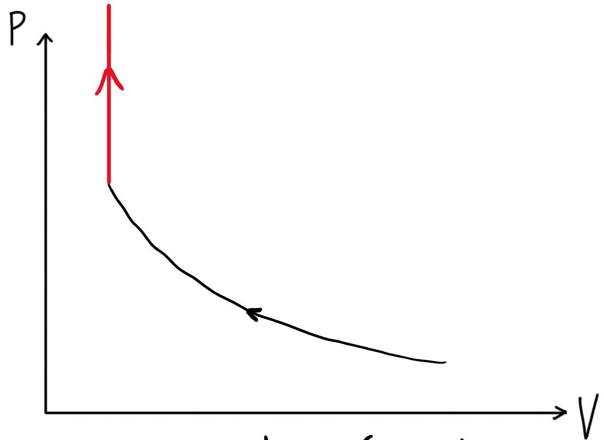
Step 2: combustion of gasoline
