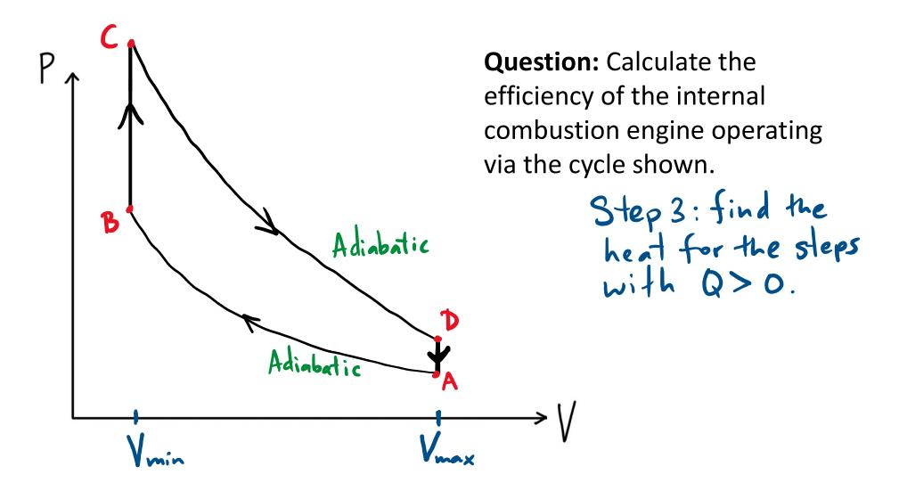
Calculate Q for the process B -> C: const. volume : W = O
