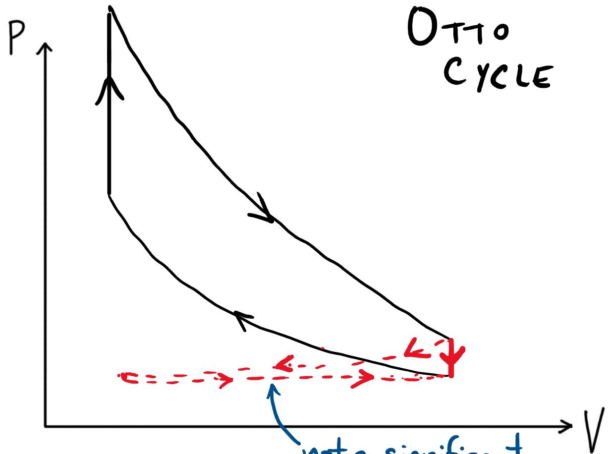
not a significant amount of net work, so model as constant volume process
