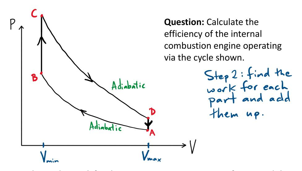
What is the work for the processes C -> D in terms of n,  $C_{V}$ , and the various temperatures, volumes or pressures?
