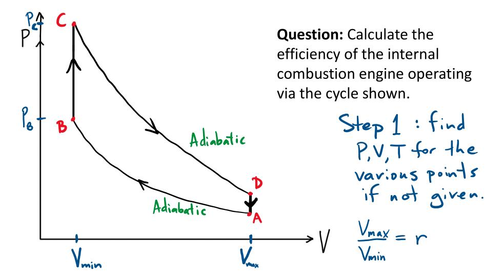
What are the temperatures  $T_B$ ,  $T_C$ , and  $T_D$  in term of  $T_A$ ,  $r = V_{max} / V_{min}$ , and  $x = P_C / P_B$
