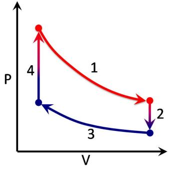
In the picture, process 1 and 3 are isothermal. During how many of the four processes does (positive) heat flow in to the gas?
