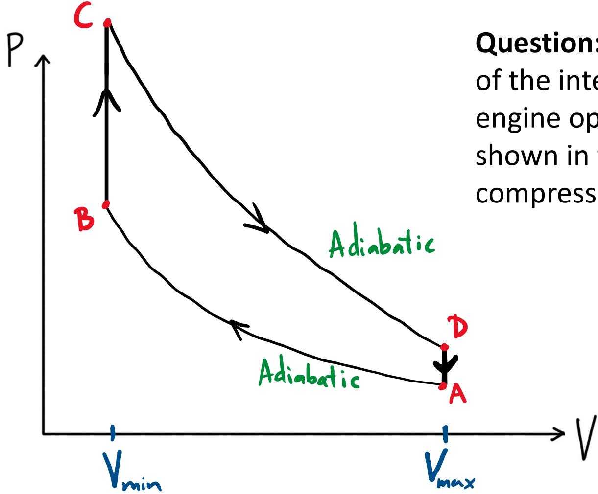
**Question:** Calculate the efficiency of the internal combustion engine operating via the cycle shown in terms of the compression ratio  $r = V_{max} / V_{min}$
