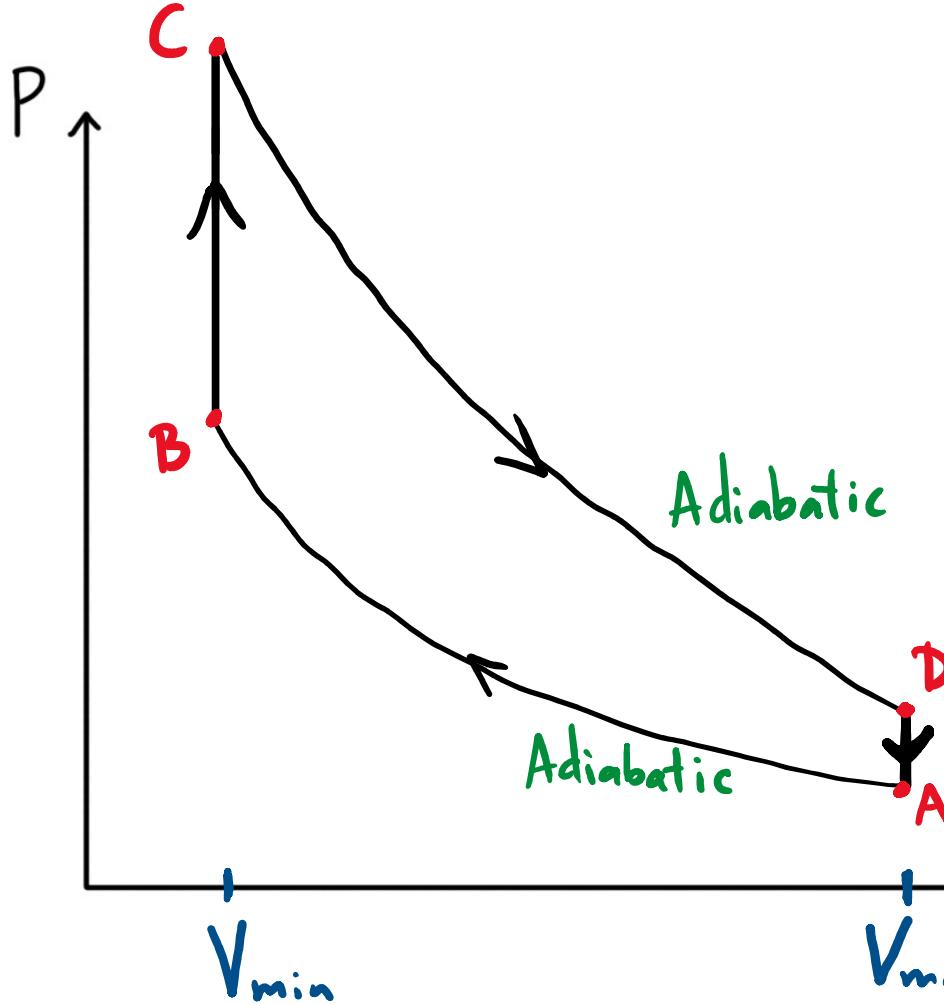
**Question:** Calculate the efficiency of the internal combustion engine operating via the cycle shown.
