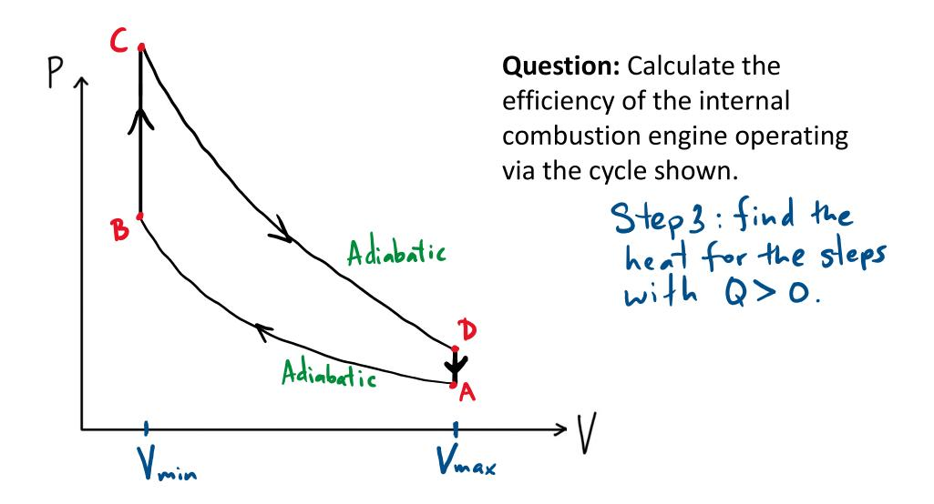
Calculate Q for the process B -> C, in terms of n,  $C_V$  and the various temperatures, pressures, and volumes.
