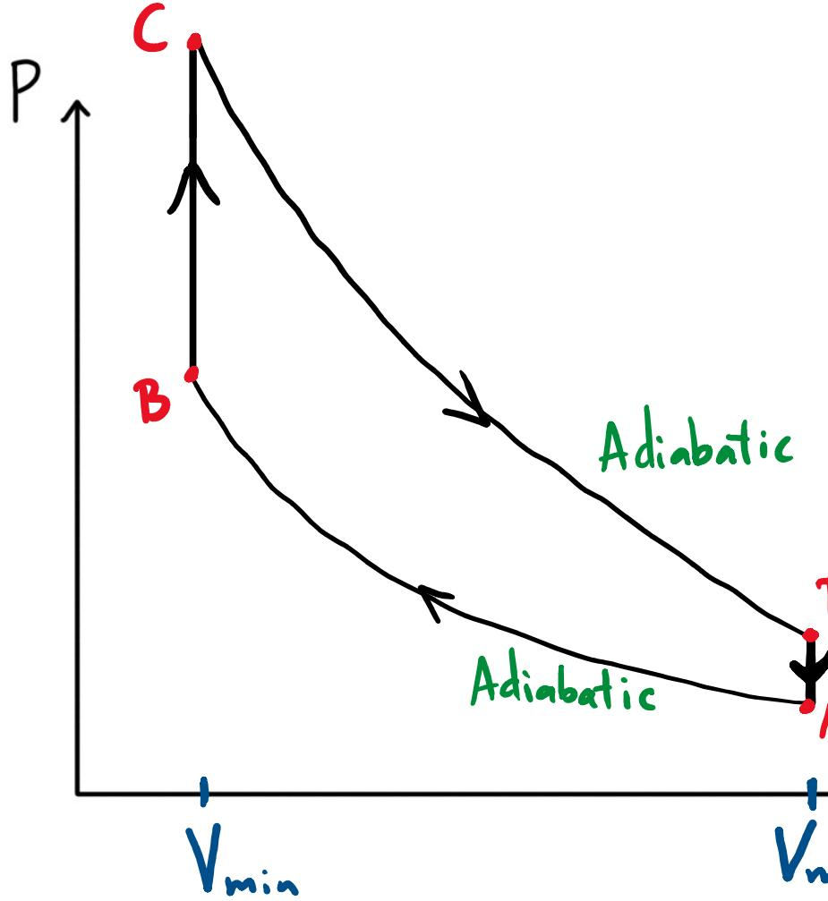
**Question:** Calculate the efficiency of the internal combustion engine operating via the cycle shown.
