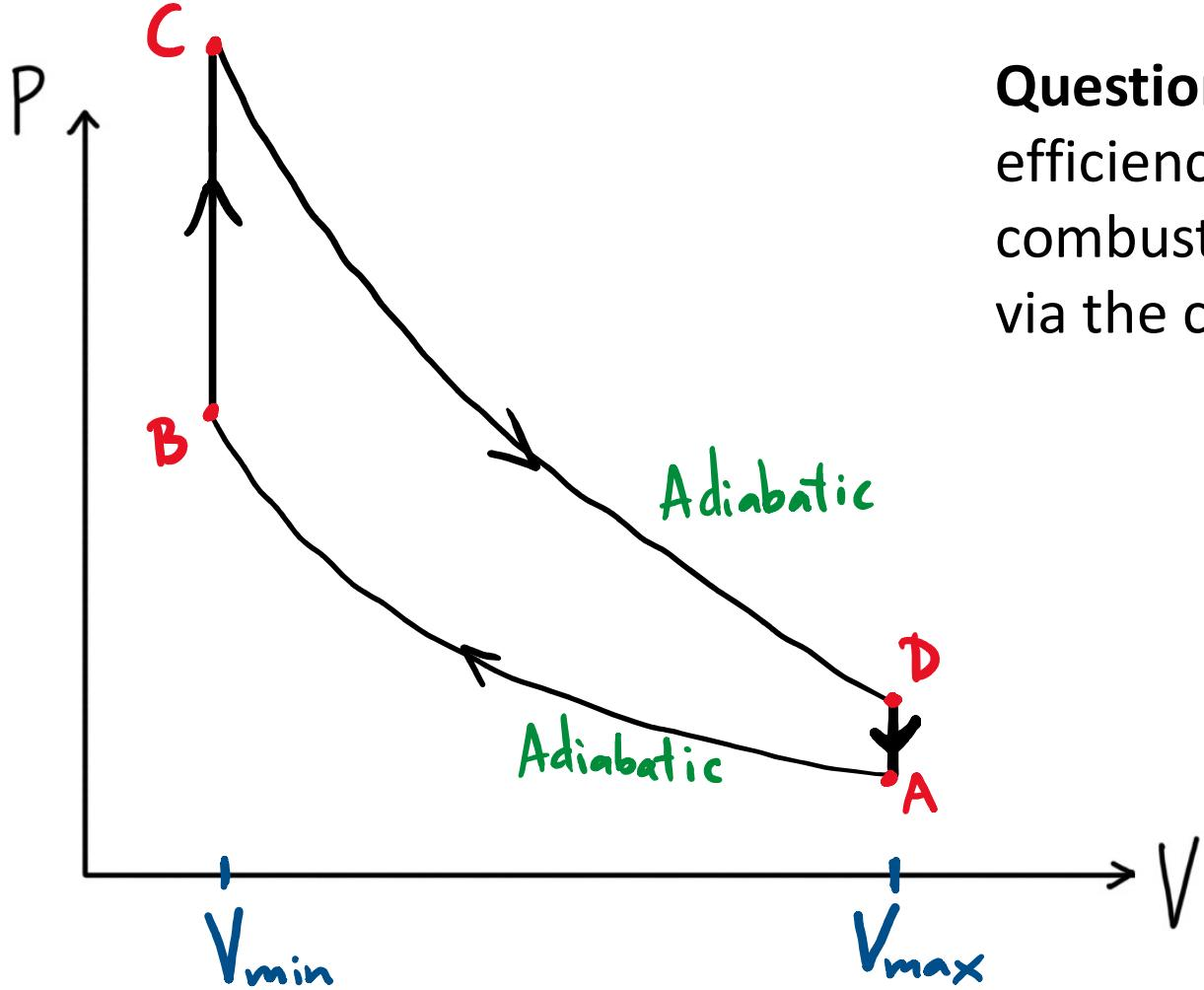
**Question:** Calculate the efficiency of the internal combustion engine operating via the cycle shown.
