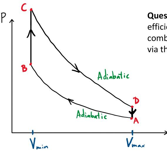
**Question:** Calculate the efficiency of the internal combustion engine operating via the cycle shown.
