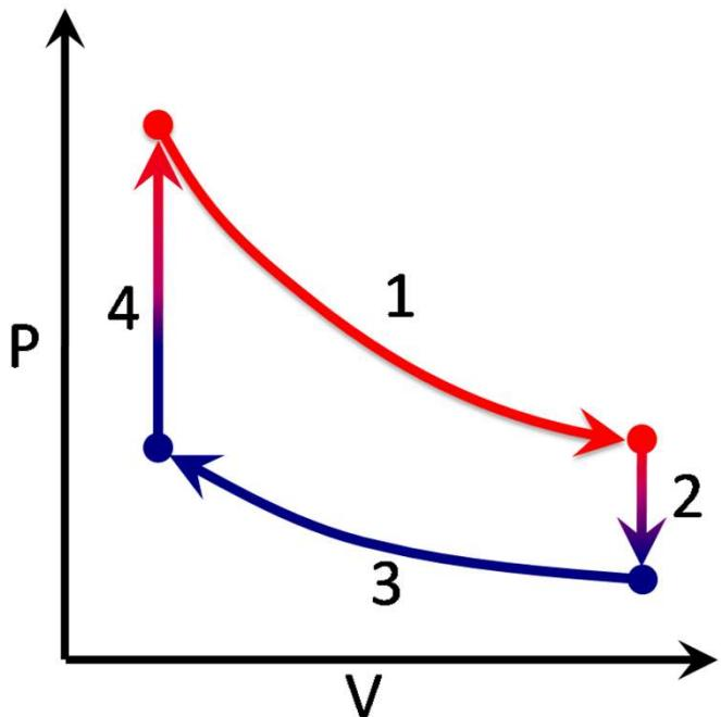
In the picture, process 1 and 3 are isothermal. During how many of the four processes does (positive) heat flow in to the gas?
