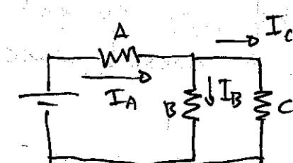
$$I_A = I \quad \text{resistance is equal, half the current goes each way.}$$
