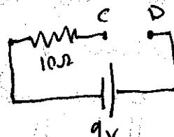
No current flows, so there is no potential drop across the 10Ω resistor ( $V = IR = 0$ ).
