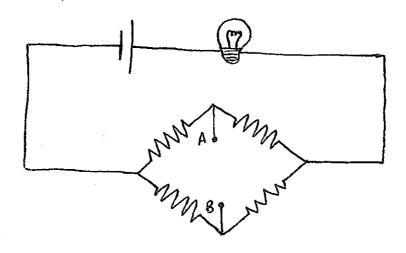
In the circuit shown above, a new resistor is added between points A and B. Does the light bulb get brighter, dimmer, or stay the same? Check your prediction. Explain the result.
