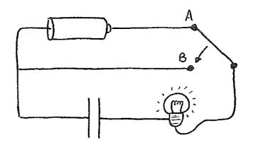
The circuit shown above includes a light bulb, a battery, and a capacitor. Predict what will happen when the switch is moved from A to B. Check your prediction using the real circuit components. Explain why the process you observe is not instantaneous, and explain how you could estimate the amount of time it takes based on the capacitance (how much charge there is on the capacitor for a given voltage) and the resistance of the bulb.
