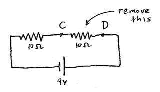
In the same circuit from problem 2 (shown schematically above) what is the potential difference between points C and D? Predict what the potential difference will be after you remove the indicated resistor. Use the simulator to check your result. Explain this result.
