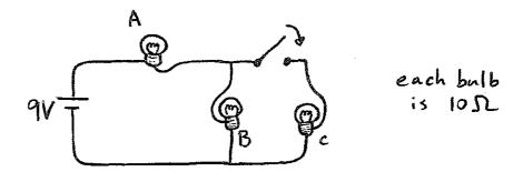
In the circuit shown, predict what will happen to the brightness of bulb A when the switch is closed. Test your prediction with the simulator. Explain the results.
