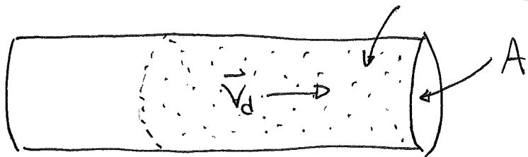
The number of electrons that pass through A after time  $\Delta t$  is
