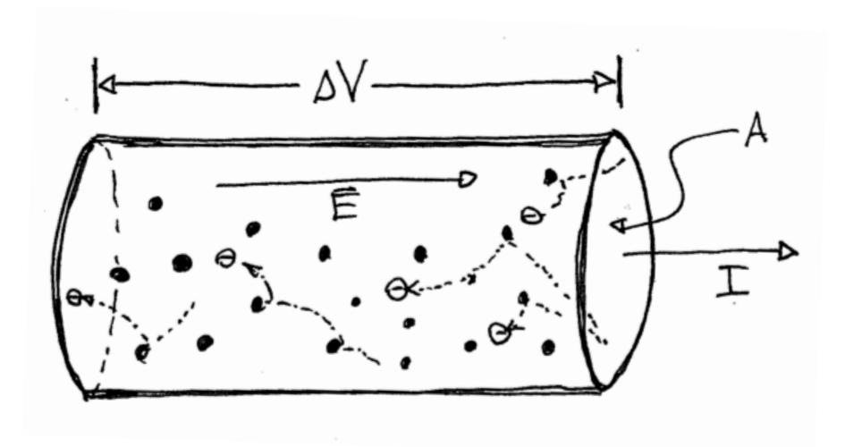
Higher voltage leads to a larger electric field and an increase in drift speed and and increase in current.
