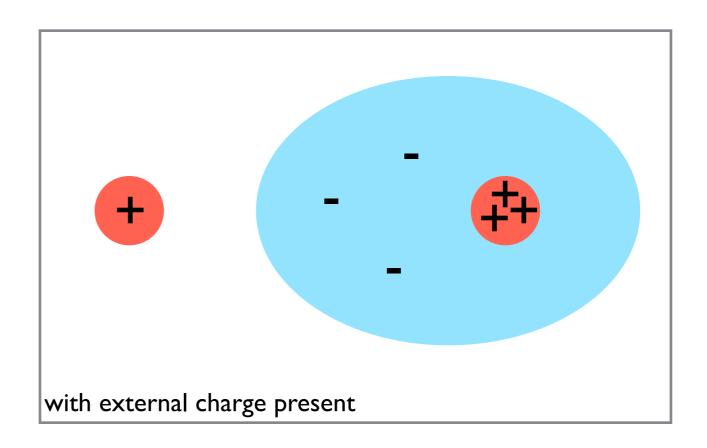
This is how the bits of paper get attracted by the balloon. The polarized atom now attracts the positive charge.
