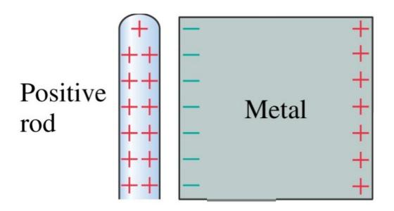
In this case the charge is free to move right to the boundaries of the material.
