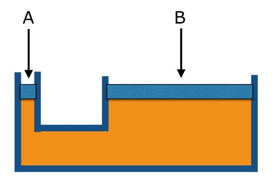
A container of gas with uniform pressure has a large piston and a small piston attached to it. The forces A and B act on the pistons from the outside such that the system is in equilibrium. We can say that
