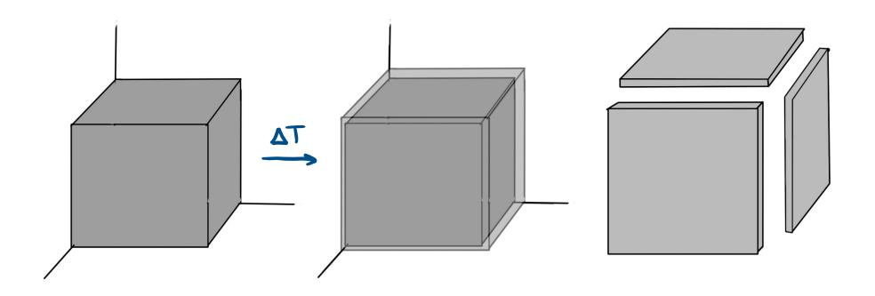
Clicker: When heated, each side of a cube of material expands by 0.1%. As a percentage of the original volume of the cube, the extra volume (shown in the third picture) after the expansion is
