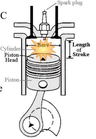
**Clicker:** In some car engines, the piston is aluminum  $(\alpha = 2.4 \times 10^{-5})$ , while the cylinder is cast iron  $(\alpha = 1.2 \times 10^{-5})$ . If the engine needs to operator between 0°C and 120°C, which of these is not a good design:
