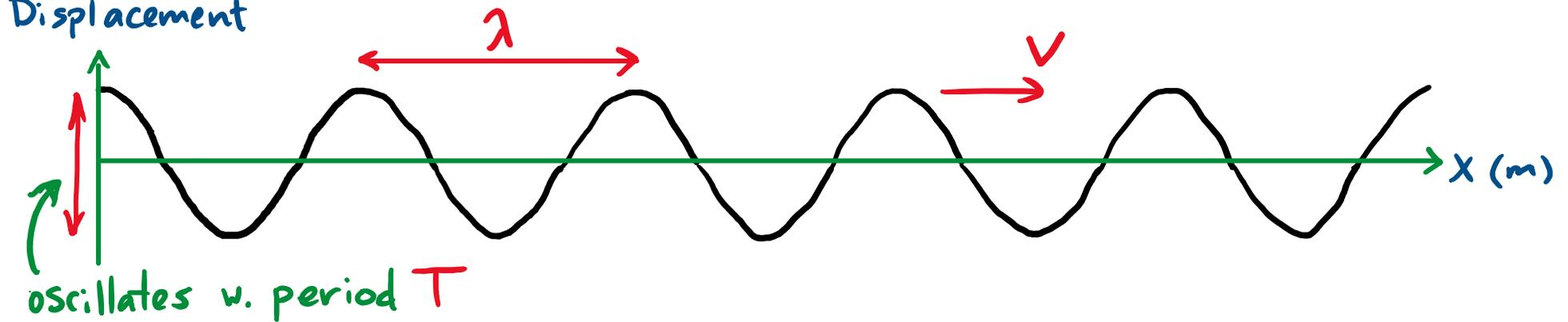
$$v = \frac{\lambda}{T} \quad \text{or} \quad v = \lambda \cdot f \quad \text{or} \quad v = \frac{\omega}{k}$$
