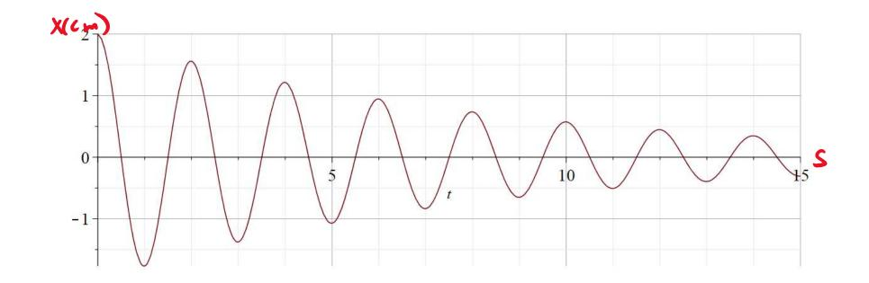
An object with mass 2kg oscillates on a spring with a small amount of damping.
