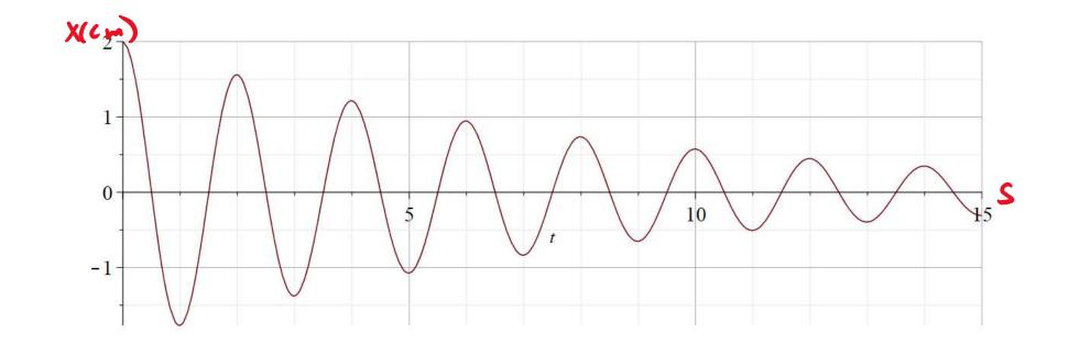
An object with mass 2kg oscillates on a spring with a small amount of damping. T = 2s so  $w = \frac{2\pi}{T}$ a) What is the damping constant b? hse  $\omega = \sqrt{\frac{k}{m} - \frac{b^2}{4m^2}}$  $= \frac{1}{2} k = m \omega^{2} + \frac{b^{2}}{4m}$  $= \frac{1}{2} \frac{N}{m} + 0.03 \frac{N}{m} \approx \frac{19.2 \frac{N}{m}}{m}$ EXTRA: What is the spring constant k? A accurate to just use  $\omega = \int_{m}^{E} unless highly damped.$
