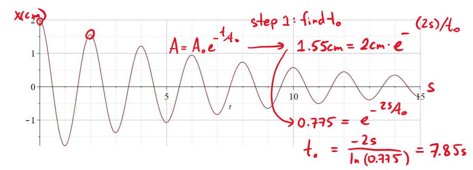
An object with mass 2kg oscillates on a spring with a small amount of damping.
