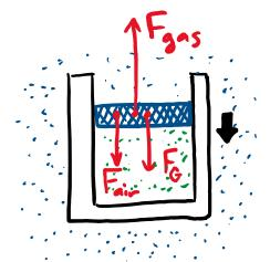
What happens to the forces if we move the piston upward a little (assume the cylinder is insulated)?
