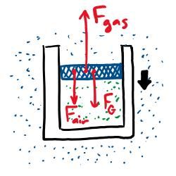
What happens to the forces if we move the piston downward a little (assume the cylinder is insulated)?
