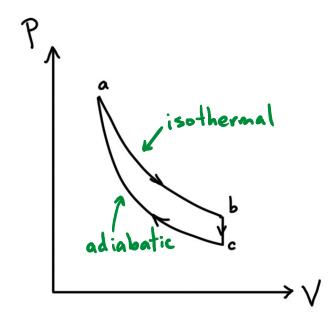
In the cycle shown, heat Q enters the gas in the isothermal step a -> b at temperature T. The entropy change from b -> c is
