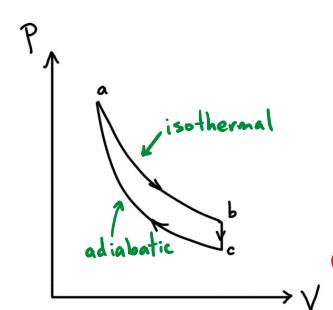
In the cycle shown, heat Q enters the gas in the isothermal step a -> b at temperature T. The entropy change during this step
