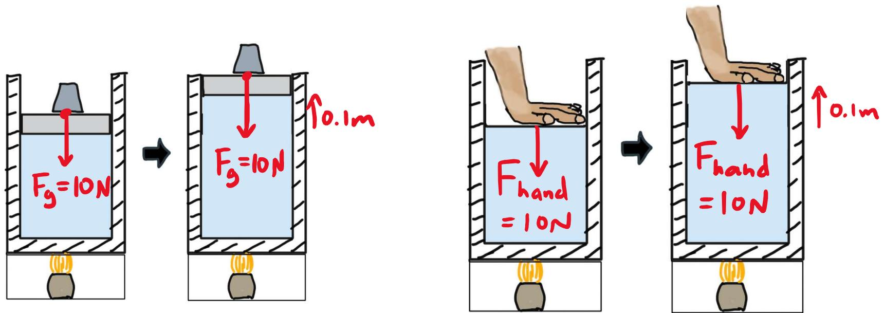
In the second picture, the hand exerts a constant 10N force opposing the expansion of the gas. The person uses up 2J of energy in order to exert this force. We can say that the work done by the gas is
