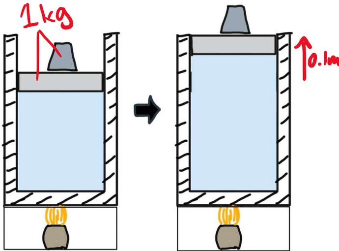
The picture shows gas in a cylinder with a movable piston on top. There is **no air** outside the cylinder. Heat 10J flows into the gas via a burner at the bottom, causing the piston to move 0.1m upwards. If the piston plus the weight on top have a mass of 1kg, by roughly how much does the energy of the gas change during this process?
