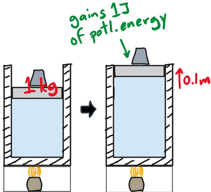
The gas did  $\sim 1\text{J}$  of work on the piston.
