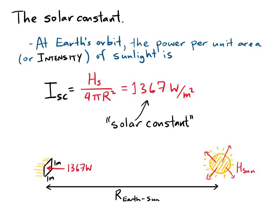
The heat current into the earth due to sunlight is  $H_{1} = \pi r^2 (1-\alpha) \mathbf{I}_{sc}$
