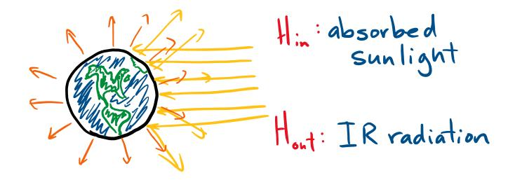
The heat current into the earth due to sunlight is  $H_{in} = \pi r^2 (1-\alpha) \mathbf{I}_{sc}$
