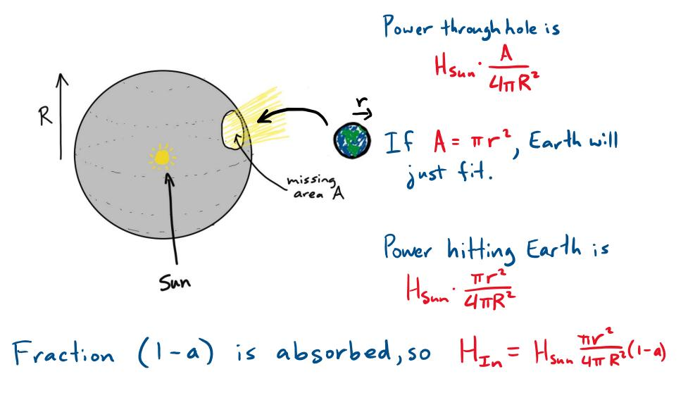
What is the power  $H_{ln}$  of solar radiation absorbed by the Earth? Answer in terms of  $H_{Sun}$ , the albedo **a** (fraction of sunlight reflected) and the parameters r and R shown below.
