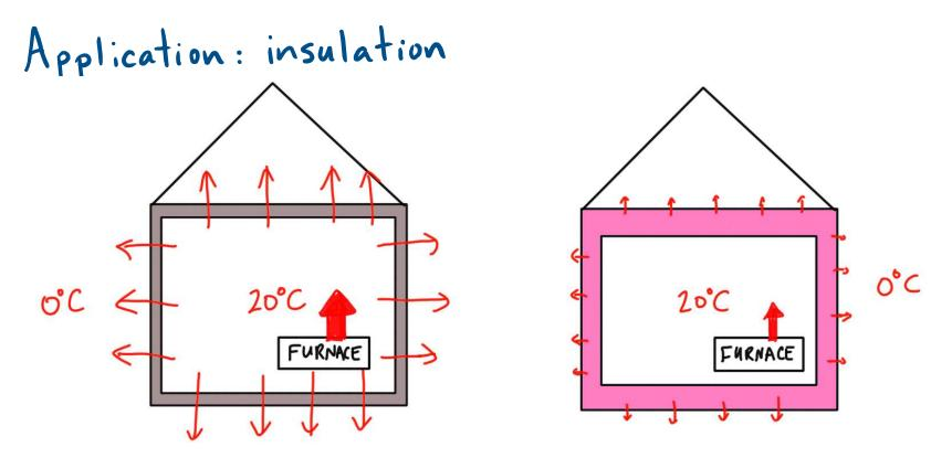
The second house has insulation that is twice as thick and made with a material that has half the thermal conductivity. To maintain the same inside temperature, the amount of fuel needed to be burned by the furnace in the second house is:
