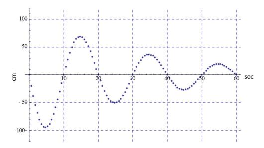
The graph shows the displacement vs time for a large object of mass 1000kg oscillating on a giant spring.
