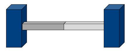
$\alpha_{\text{steel}} = 12 \text{ x } 10^{-6} \text{ K}^{-1}, \ \alpha_{\text{copper}} = 17 \text{ x } 10^{-6} \text{ K}^{-1},$  $Y_{\text{steel}} = 200 \text{ x } 10^9 \text{ N m}^{-2}, \ Y_{\text{copper}} = 110 \text{ x } 10^9 \text{ N m}^{-2}$
