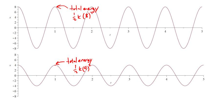
The two graphs show different oscillations for the same system. Compared with the first case, the total potential plus kinetic energy in the second case is
