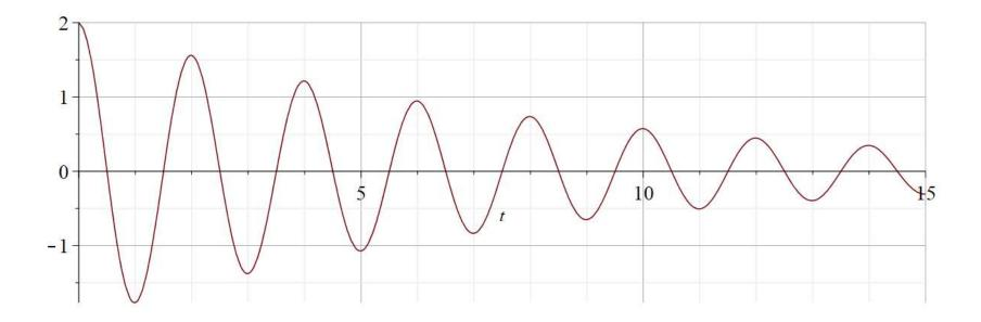
EXTRA: An object with mass 2kg oscillates on a spring with a small amount of damping.
