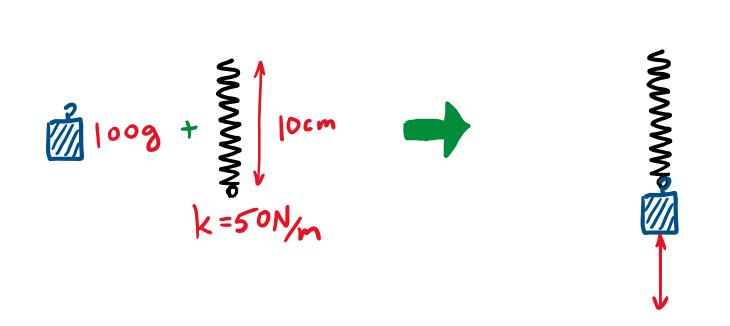
**Discussion question:** A 10cm long spring has a spring constant of 20 N/m. If we attach a 100g weight to the spring and release it, what will be the amplitude of the resulting oscillation?
