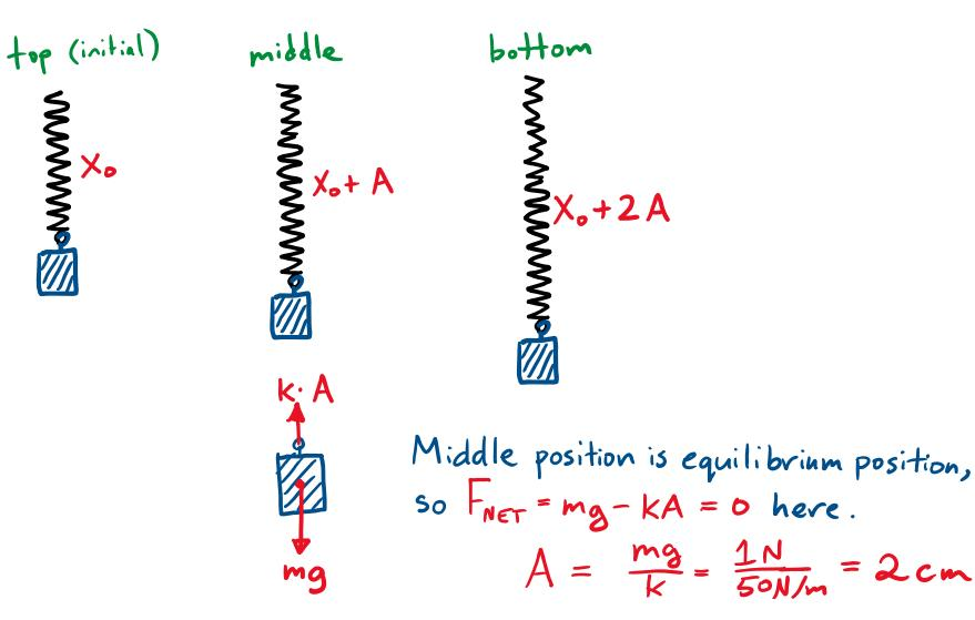
How to find  $\omega$  in examples: 1) Find FNET as a function of position x FNET Find equilibrium value Xeq by solving Fret (X.) = 0. 3 - k is FNET (Xeq), the slope at Xeq. slope here
