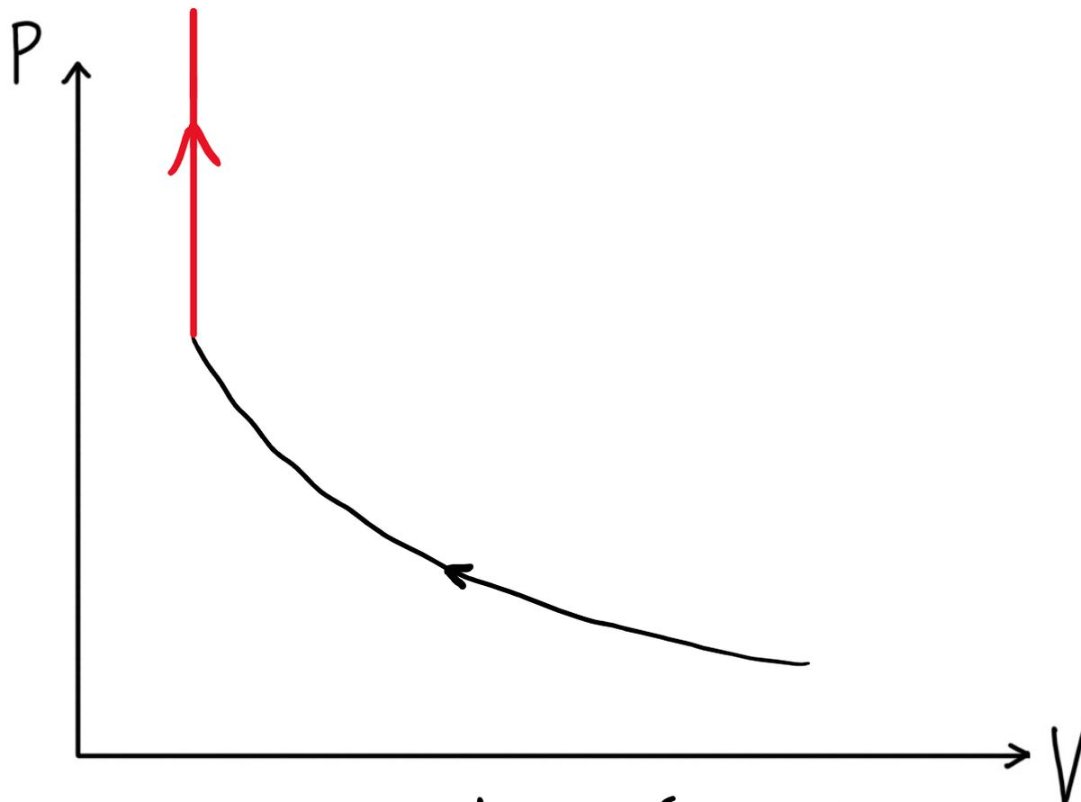
Step 2: combustion of gasoline
