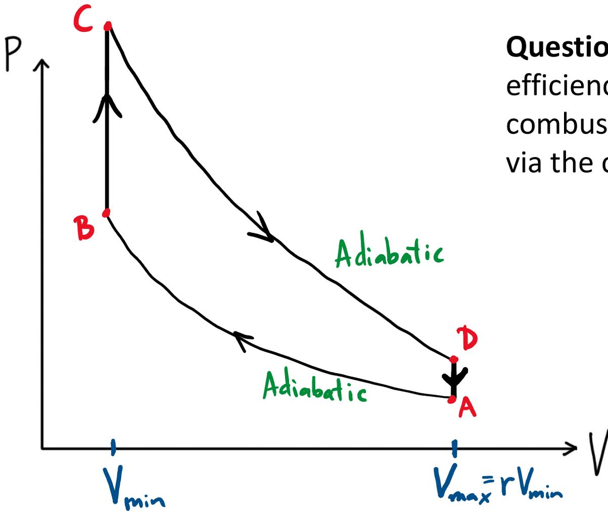
**Question:** Calculate the efficiency of the internal combustion engine operating via the cycle shown.
