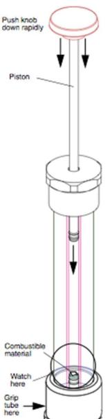
Demo: we can ignite cotton just by compressing the air!
