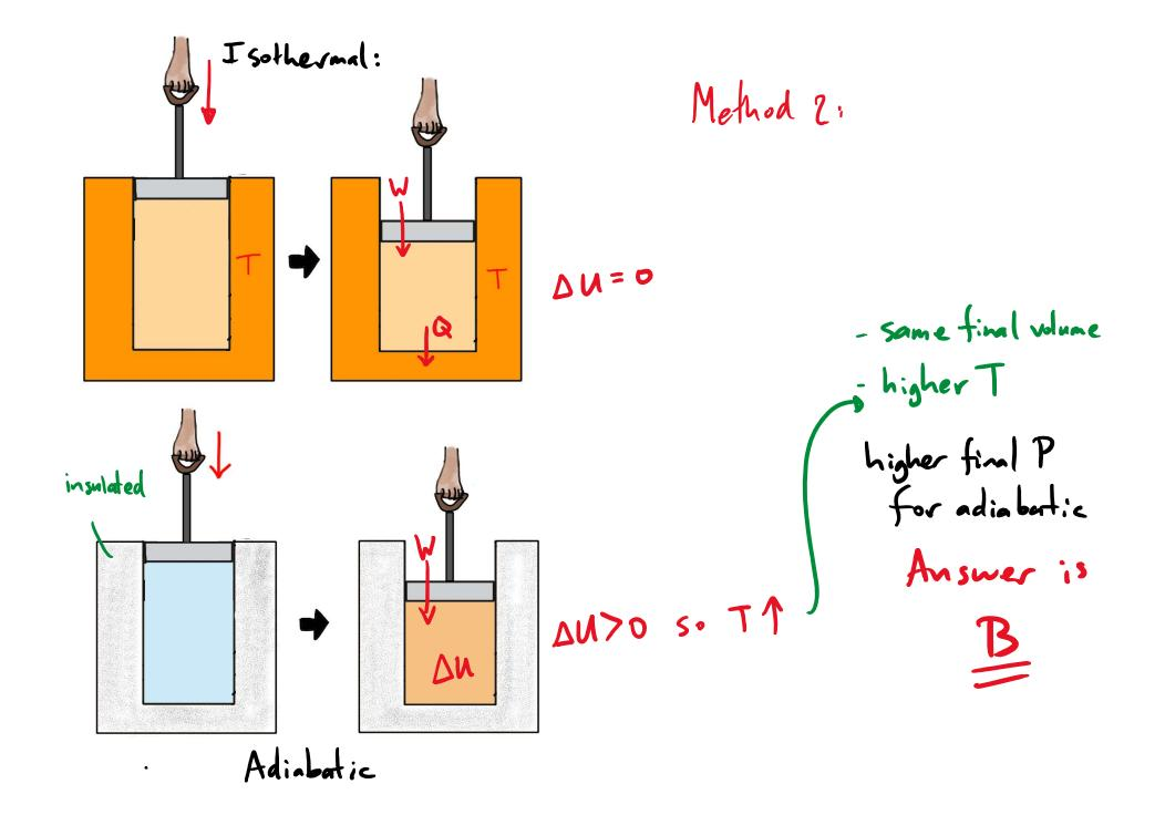
Gas with  $C_V = 3$  R, initially at room temperature, is compressed very rapidly in a cylinder. The **compression ratio** is 15.
