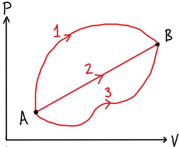
The graph shows three possible processes for an ideal gas going from A to B. For which path is Q (the heat added) the largest?
