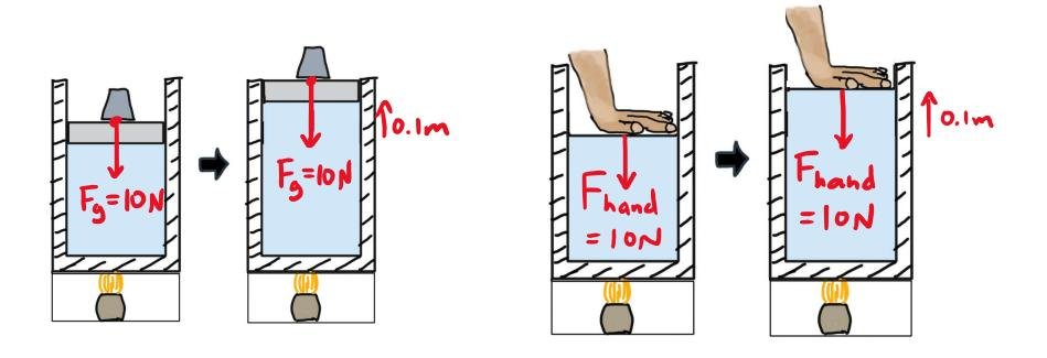
In the second picture, the hand exerts a constant 10N force opposing the expansion of the gas. The person uses up 2J of energy in order to exert this force. We can say that the work done
