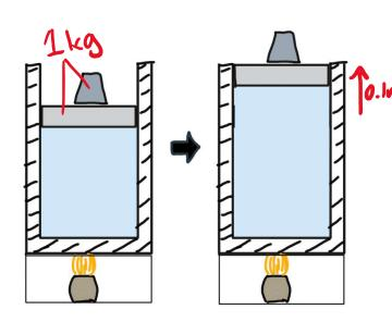
The picture shows gas in a cylinder with a movable piston on top. There is no air outside the cylinder. Heat 10J flows into the gas via a burner at the bottom, causing the piston to move 0.1m upwards. If the piston plus the weight on top have a mass of 1kg, by roughly how much does the energy of the gas change during this process?
