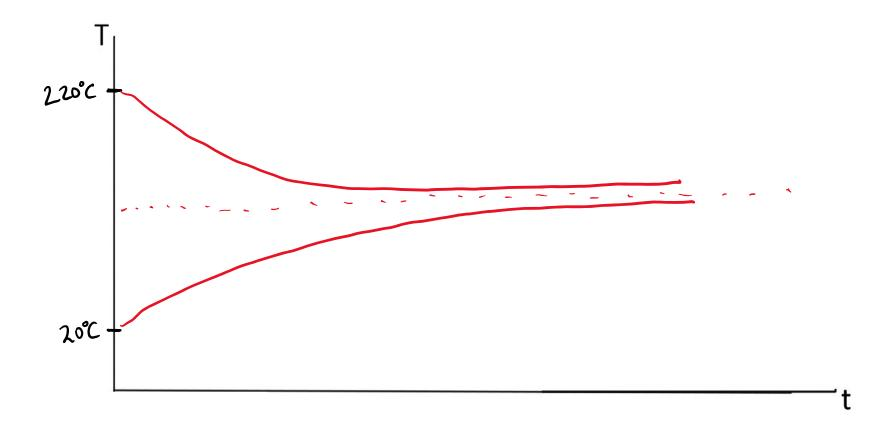
$$T_{H} = 220^{\circ}C \qquad A \\ J k \qquad T_{c} = 25^{\circ}C \qquad C = 900 \ J/kg \\ k = 200 \ W \cdot K \\ k = 200 \ W \cdot K \\ A = 0.1 cm^{2} \\ L = 1 cm$$
