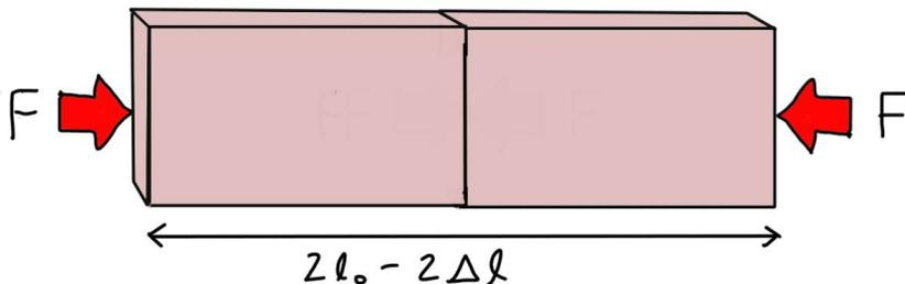
If we double the cross-sectional area of the block, we'll need twice as much force to get the same compression, since this situation is equivalent to having two of the original blocks side by side as shown. So the constant  $C$  should double.
