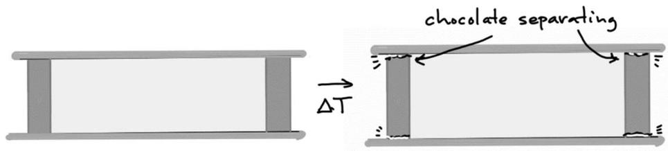
b) After the graham crackers are attached, and the entire cookie is in equilibrium at  $10^{\circ}\text{C}$ , there is no stress in the marshmallow or chocolate. The chocolate will separate from the graham cracker if the (vertical) tensile stress in the chocolate exceeds  $1.3 \times 10^3 \text{ Pa}$ . What is the maximum temperature increase the cookies can withstand without the chocolate separating?
