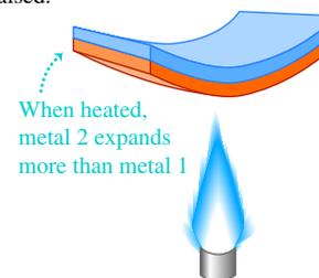
(c) A bimetallic strip used in a thermometer
