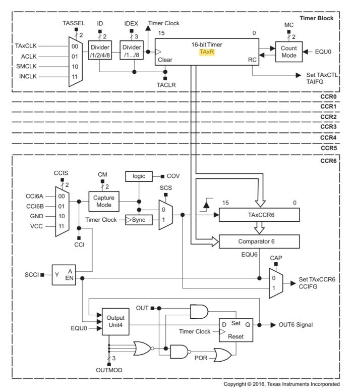
Figure 17-1. Timer\_A Block Diagram
