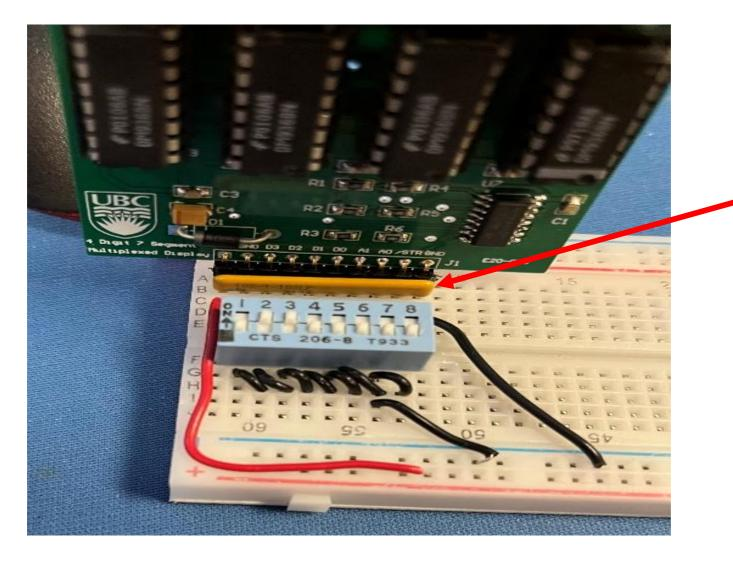
resistor block With pin 1 on the left connected to red wire
