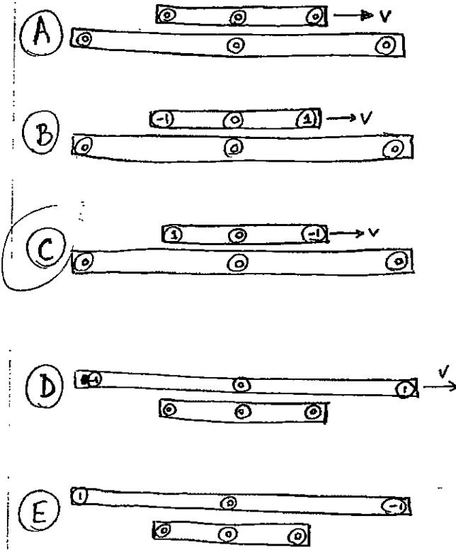
Two identical meter sticks, each with synchronized clocks at the ends and in the middle, pass each other at  $v = \sqrt{\frac{3}{4}}c$ . Which picture represents a possible observation of the system at some instant in the frame of the lower meter stick. Numbers in the circles represent the clock readings (in some units).
