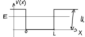
As long as the particle's energy E < U, the electron is confined to the wire. The bound states can be seen in the bound-state simulation applet. You also studied them in Tutorial 11.
