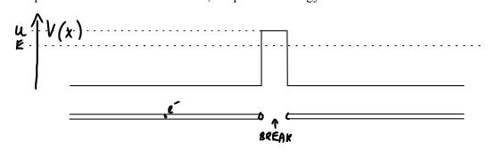
Classically an electron inside the wire with E<U cannot get over the break. In QM, it can! Current can flow across a broken wire.
