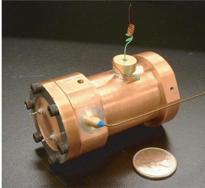
Figure 7.2: Image of the shear cell, next to a Canadian quarter for scale.
