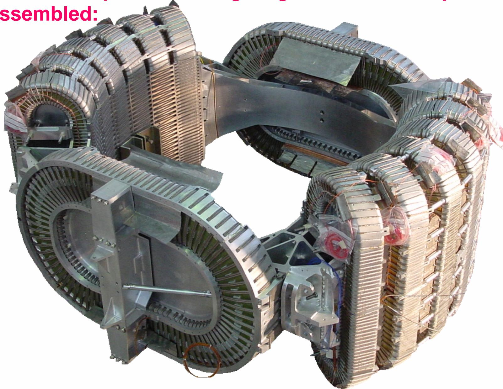
Volume 35 cu. ft., Field 8,600 Gauss, Weight 2 tons
