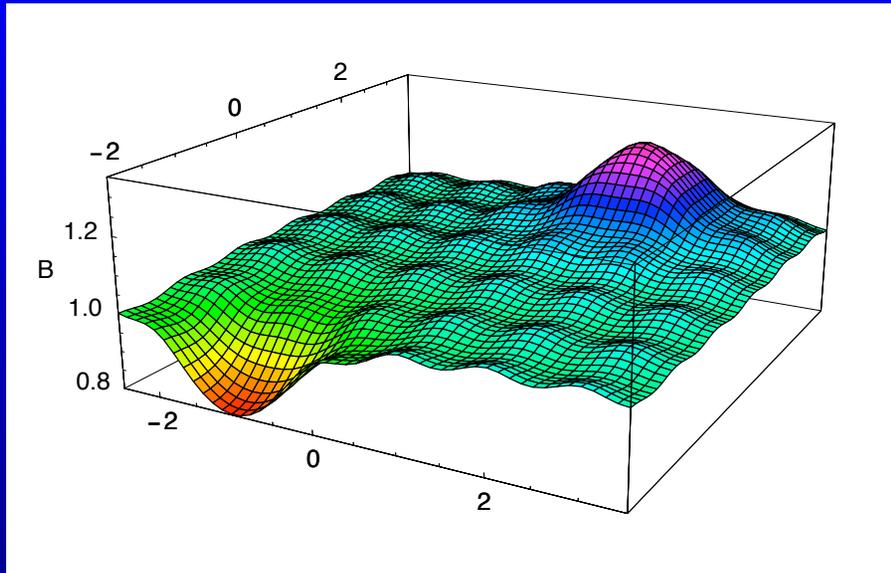
Magnetic field profile with one **vacancy** and one **interstitial**, based on a simple London model with penetration depth  $\lambda = a$  intervortex spacing.
