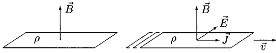
FIG. 2. When a disorder-free 2-d electron gas is placed in a magnetic field it can be Lorentz boosted to generate a current and a transverse electric field. The ratio of these then gives Eq. (3), which is inconsistent with all quantum Hall experiments. This shows that disorder is essential for plateau formation.
