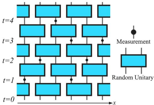
FIG. 2. The random circuit model. This circuit displays the commonly used brick-layer pattern for random unitaries with single-qubit measurements randomly interspersed between the unitaries. The measurements are randomly placed with a Poissonian distribution, where each position and time combination has a probability  $p$ . The total number of possible combinations is simply the number of positions multiplied by the depth.
