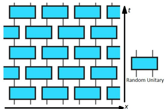
FIG. 1. The random circuit model. This circuit displays the commonly used brick-layer pattern for random unitaries. Notice that the above circuit shows both spatial symmetry, with a lattice constant  $a$ , and temporal symmetry, with a time constant  $2\tau$ .
