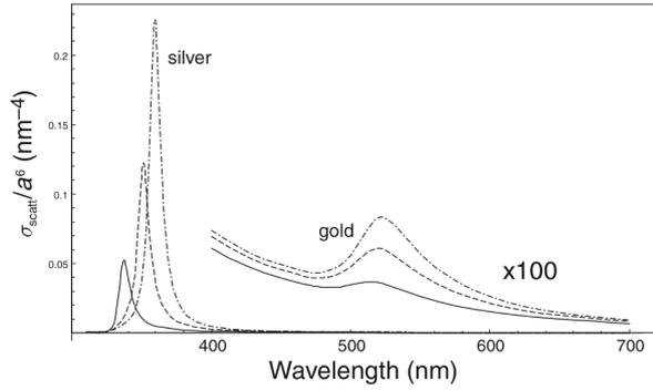
**Figure 2:** Scattering cross section of a gold or silver nanosphere following excitation with a plane wave, with the surrounding medium being  $n=1$  for a vacuum (solid),  $n=4/3$  for water (dashed),  $n=3/2$  for glass (dash-dotted). Taken out Fig. 12.22 [2]
