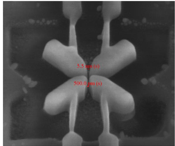
**Figure 5:** Crossed nano-antenna with a gap of 5 nm [8]
