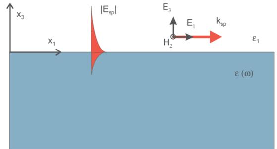
**Figure 1:** A schematic sketch of surface plasmon polaritons propagation on an interface. Taken out of Fig.1 [1]
