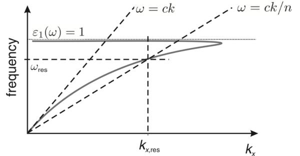
**Figure 4:** Dispersion relations of light in a vacuum and a high refractive medium. The intersections with dispersion curve of the surface plasmon polaritons show a clear excitation frequency. Taken out Fig. 12.8a [2]
