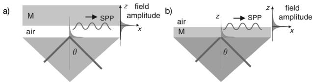
**Figure 3:** a) is the Otto configuration and b) the Kretschmann configuration. In both cases **M** denotes the metal. The light beam under the critical angle  $\theta$  in the high refractive medium is shown in dark grey. Taken out Fig. 12.8b-c [2] and added.
