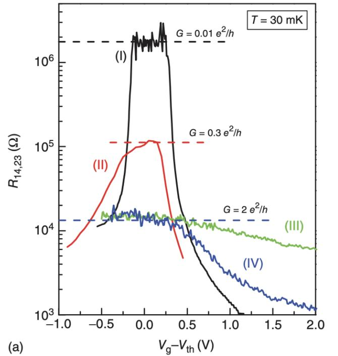
FIG. 4: Transport measurement of CdTe/HgTe/CdTe quantum wells of varying thickness. Samples (III) and (IV) have thicknesses past the critical topological phase transition value and are found to have the theoretical longitudinal conductivity of  $G = 2 \cdot \frac{e^2}{2\pi\hbar}$ . This figure demonstrates the first experimental evidence of a TI phase. Figure taken from [5].
