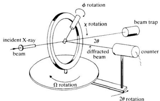
FIG. 3. 4-circle goniometer, to rotate the sample freely about any axis [1].
