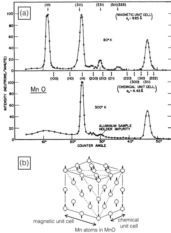
FIG. 6. (a) Neutron diffraction patterns for MnO at 80 K and at 300 K. At low temperature, four extra diffraction peaks appear. (b) Chemical and magnetic unit cell of MnO [12].
