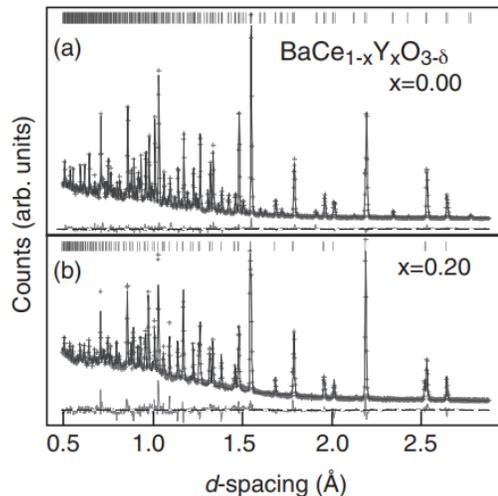
FIG. 2. Observed diffraction intensities for BCY at room temperature, with  $\delta = x/2$ . A difference curve between observed and calculated intensity is shown below each profile [5].
