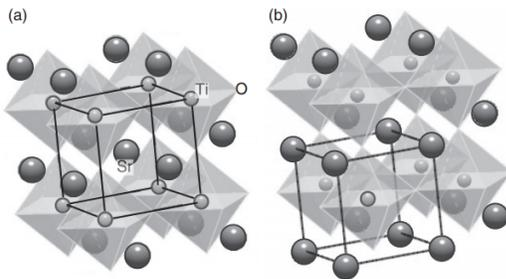
FIG. 1. The idealized perovskite structure of  $\text{SrTiO}_3$ . The solid lines outline the primitive cubic unit cell [5].
