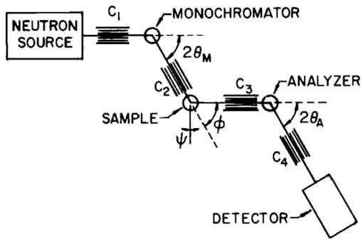
FIG. 4. A diagram of a triple-axis spectrometer [11].
