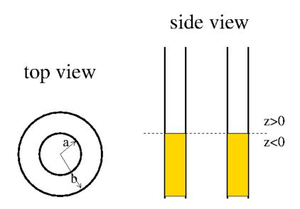
10. A dielectric fluid ( $\epsilon > \epsilon_0$ ) fills the space between two infinitely long concentric, perfectly conducting cylinders for z < 0. The region z > 0 between the cylinders is open to the atmosphere ( $\epsilon = \epsilon_0$ ). The cylinders have radii a and b and are sufficiently long that edge effects can be neglected. The inner cylinder is charged to potential  $\Phi = V > 0$ , while the outer cylinder is grounded at  $\Phi = 0$ .
