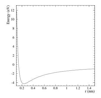
4. A NaCl molecule has an ionic bond between a Na<sup>+</sup> and a Cl<sup>-</sup> ion. The potential for this system as a function of r, the distance between the ions, may be described by:
