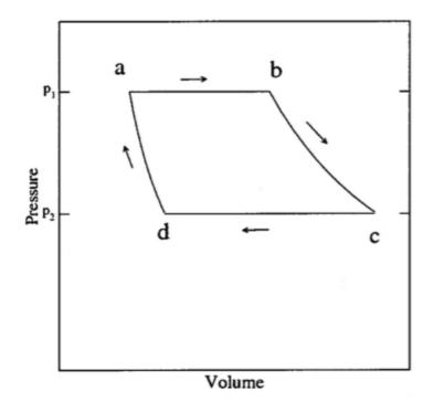
12. An ideal gas of N molecules, each with g degrees of freedom, is carried around the reversible closed cycle shown above. Two of the segments are adiabatic, and two are isobaric (constant pressure).
