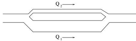
The pipe carrying flow  $Q_1$  has a radius of  $R_1$ , and the pipe carrying flow  $Q_2$  has a radius of  $R_2$ . Derive the effective impedance of this ensemble of pipes, again ignoring end effects. Show that the impedance of the combination has the same relation to the individual impedances of the two pipes as the resistance of two electrical resistors in parallel has to their individual resistances.
