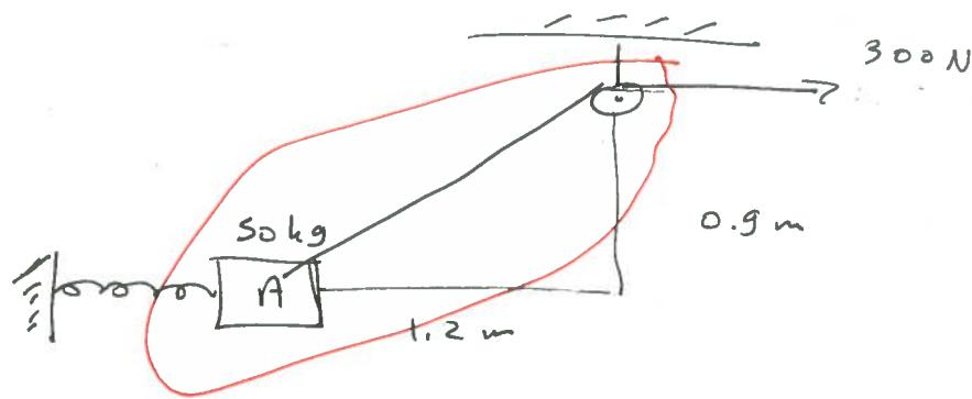
The system we are considering is encircled. The force the pulley and A exert on each other is equal and opposite in direction, so that part of the work cancels.
