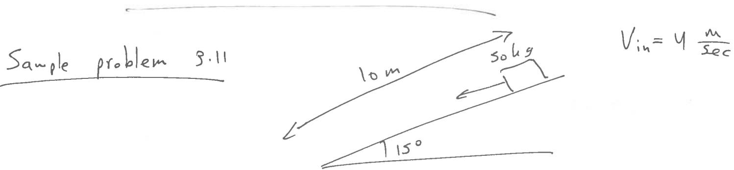
Calculate final velocity when crate reaches bottom. Coeff.
